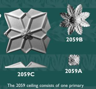
The 2059 ceiling consists of one primary component, the 2059C border piece, and two optional rosettes: the 2059A and 2059B. The principal piece measures 31<sup>1</sup>/4 inches (794 mm) square. 16 pieces cover 108 sq. ft (10.1 sq. m).
