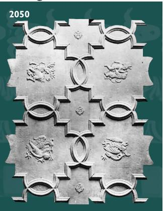
The 2050 ceiling consists of six component parts: the H-shaped 2050B plus five ornamented infils. Components are laid out on a 411/4 inch (1.05 m) grid. To cover 100 sq. ft (9.29 sq. m), 36 pieces are required plus cutting allowance.
